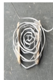
(Fig 2) Aluminum wire electrodes
