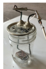
(Fig 1) 1.5 -12-volt battery hooked up to a metal wire for electrolysis
