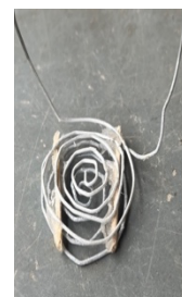
(Fig 2) Aluminum wire electrodes
